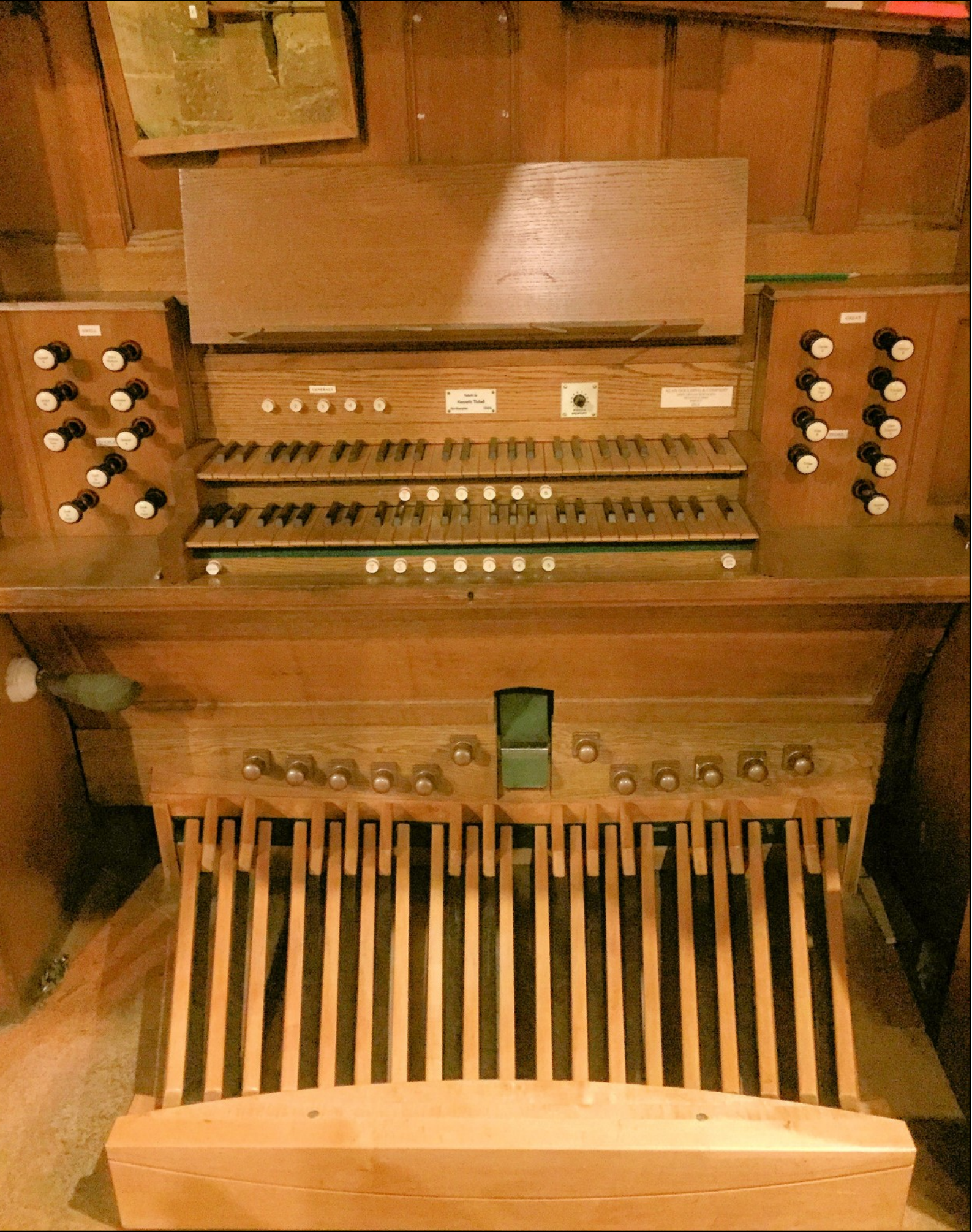
The console of St. John the Baptist, Kingsthorpe following fitting of electric draw-stop and piston mechanisms ( Picture by Andrew Moodie ).
